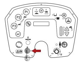
Press the brush attach/release button; the machine will respond by operating the release mechanism.
