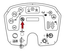
Select the type of batteries installed using the "+" or "-" button: "ACID battery" or "GEL battery".
