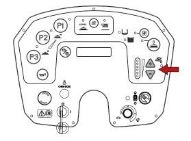
Chem Dose model, press the switch to turn on the device. To change the percentage dilution of the detergent (Chem Dose model), refer to the section "Selecting the percentage dilution of the detergent (Chem Dose model)".
