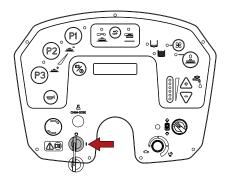
Press buttons "1 and 3" at the same time, then switch the machine on by turning the ignition key.
