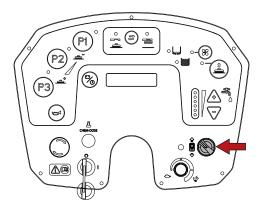
Roller head model: lower the side brushes by pulling and lowering the levers. The brush motors will come into operation only when the brushes are completely lowered.
