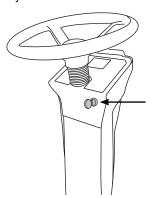
Press the AUTO or ECO button; in both modes, all the machine's functions will be activated. In ECO mode, the machine consumes less energy and operates more silently.
