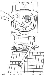
Check that the suction filter is undamaged and clean
